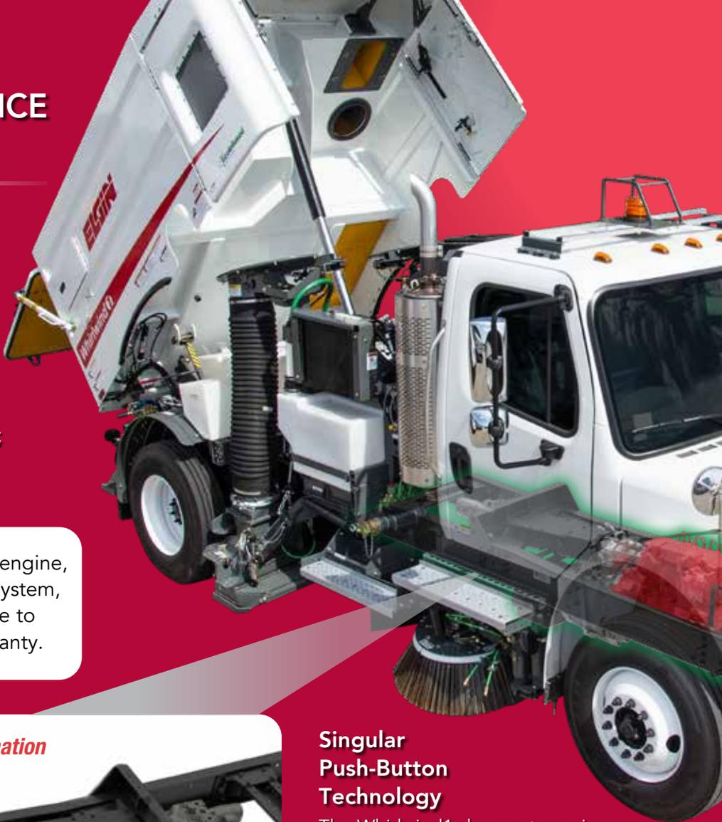
The VSD replaces the diesel auxiliary engine, eliminates a complex aftertreatment system, and untimely regenerations. It's simple to operate, and carries a three year warranty.
