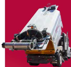
QUICK COMPLETE DUMPING 10 and 13 cubic yard (7.65 and 9.94 cubic meter) hoppers are constructed with 10-gauge steel walls and ceiling, a 1/4 inch (6.35 mm) thick floor with drop-down screens for quick cleanup.
