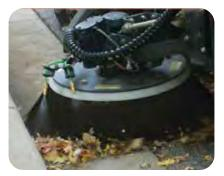
broom. The "open throat" suction nozzle design reduces clogging and plugging associated with leaves, twigs, mud, bricks and broken pavement.
