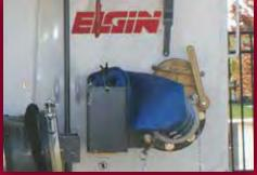
**6" DOOR DRAIN** Decanting of water aids in optimizing your payload capacity; eliminates unnecessary carrying of water weight.
