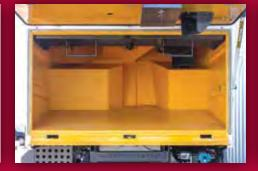
**LIFELINER® HOPPER SYSTEM** The LifeLiner® hopper liner and finish system greatly improves the life, durability, and dumping functionality of a sweeper hopper. It is backed by a lifetime warranty.\*\*
